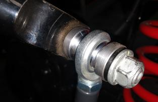
15. Assemble the front passenger side quick release clevis pin with a spring washer as shown.
