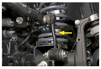
11. Remove the upper end link from the sway bar with a 6mm hex key and a 18mm wrench.
