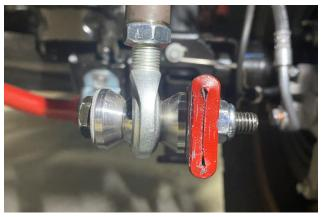
25. Slide the end link onto the clevis pin and secure with the provided quick release nut and cotter pins. The nut can be tightened by hand for easy removal on the trail, or tightened using a wrench.
