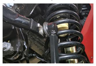
12. Place threaded pin into axle tab on driver side, facing inboard, with the cotter pin hole angled as shown. Hold the pin by the two flat surfaces to tighten the supplied nut. Place a spring washer on the pin as shown.
