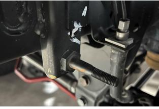
20. Remove the end links from the sway bar using a 6mm hex key and a 18mm wrench. Allow the sway bar to swing away from the workspace.
