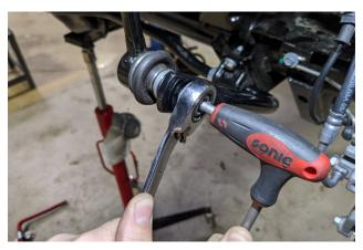
21. To install the end link disconnect holder brackets, remove the lower shock bolt, and swing the shock out of the way. Attach the bracket to the lower shock mount; place the M12 x 1.75-25mm bolt through the existing hole in the lower shock mount and fasten the bolt with the M12 flag nut from inside the lower shock mount. Leave the bracket loose until the shock hardware is tightened.
