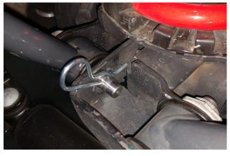
17. Slide the driver side end link onto the pin on the axle, and secure with cotter pin.
