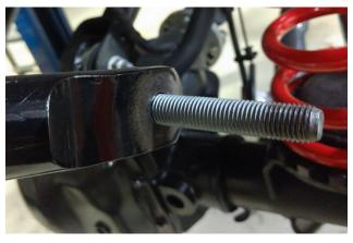
14. Install the new front end links with a cone spacer on each side of the upper Heim. Use the original lower nut on the drivers side. On the passenger side, use the supplied nylon lock nut. Torque the upper nut to 69 ft lbs. Leave the jam nut on the end link loose at this time.
